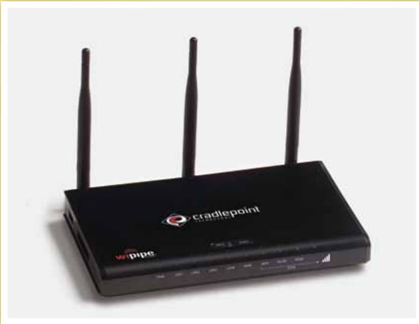
The CradlePoint MBR1000 instantly creates a Wi-Fi hotspot that any Wi-Fi enabled device can connect to—laptop, camera, PDA, etc. The MBR1000 connects devices to the Internet in two ways: via 3G/4G mobile broadband using an EVDO or USB air card, providing high-speed web access virtually anywhere. Or it can also be plugged into a DSL or cable modem.
